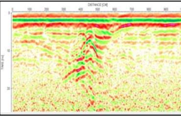
(Fig. 4b) Radargram of concrete plate using a georadar (900MHz) we found a disturbance
