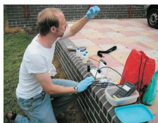
Measuring conductivity of pig carcass fluid, soil-water & basic elements, with conductivity & bulk ground resistivity (10 week) results
